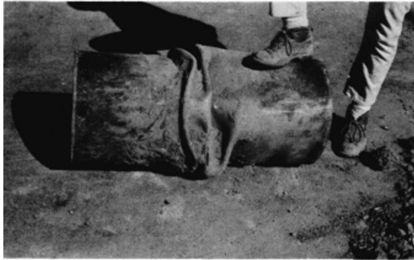
Gas pipe taken from the shear-thrust zone across Glenoaks Boulevard – USGS photo
